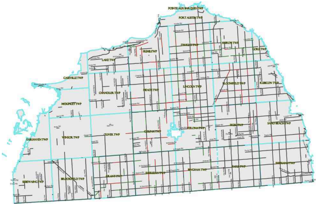
Figure 26: Map of the current IBR for drainage adequacy with good (2' or more) shown in green, fair (0.5' to less than 2') shown in orange, and poor (less than 0.5') shown in red. Only unpaved roads owned by HCRC are shown.
